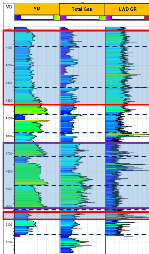
Figure 3. Surface drilling derived logs (left) validation by LWD (center) and mud logs (right). Based on the petrophysical analysis on nearby exploration well, the target formation has low GR, high YM characteristics, which are exhibited in the general trends through the comparison between drilling derived YM, LWD GR log, and Total Gas log, where low YM corresponds to low total gas and high GR (red box) and vice versa (purple box). An interesting observation is that the abrupt change of lithology and petrophysical property can be captured by the derived geomechanical log (dashed horizontal dark blue lines), which is important to well steering and completion design.
